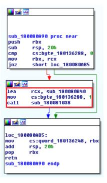
This function pointer is encoded and stored at the address *EMET64+1362a0(offset \* 8)* where *offset* is read from *EMET64+0x135320*. We can easily read these values using our read primitive to get a second pair of known encoded and plain pointers.
